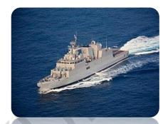
❖ The anti-submarine warfare (ASW) stealth corvettes have been undertaken under 'Project 28', also called Kamorta-class corvettes of the Navy.
